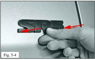
(d) Visually verify that the SR5 Emblem Cap is positioned correctly over the factory emblem and press lightly to adhere (Fig. 5-4).
